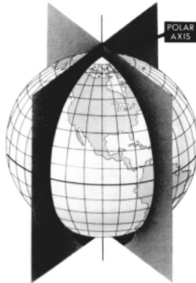
Figure 104a. The planes of the meridians meet at the polar axis.
